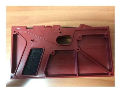
The six holes, three on the front and three on the back, are drilled into the spots marked as "M3" or "M4" on the assembly jig: $^{18}$
